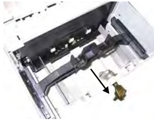
Pull the packer plate back. Cassettes allow the pusher-plate to be latched in position using the key-lock.
