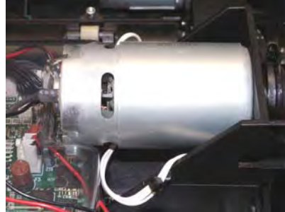
DC drive motor from TDM-1XX modified
