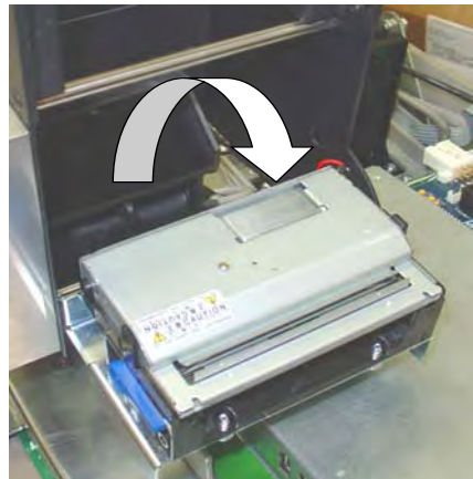
Rotate printer/cutter assembly down.
