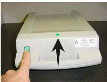
Press release button and lift top.
