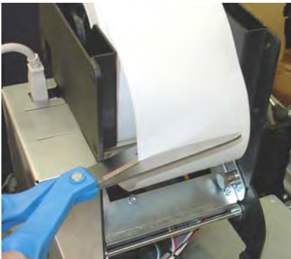
Cut paper between roll and paper path
