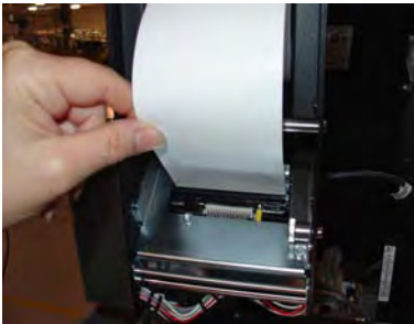
Feed paper into the printer take-up slot.
